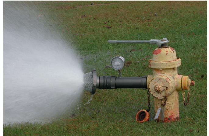
Figure 4-6. A Hydrant Being Flowed with a Diffuser as Part of a Fire-Flow Test.
